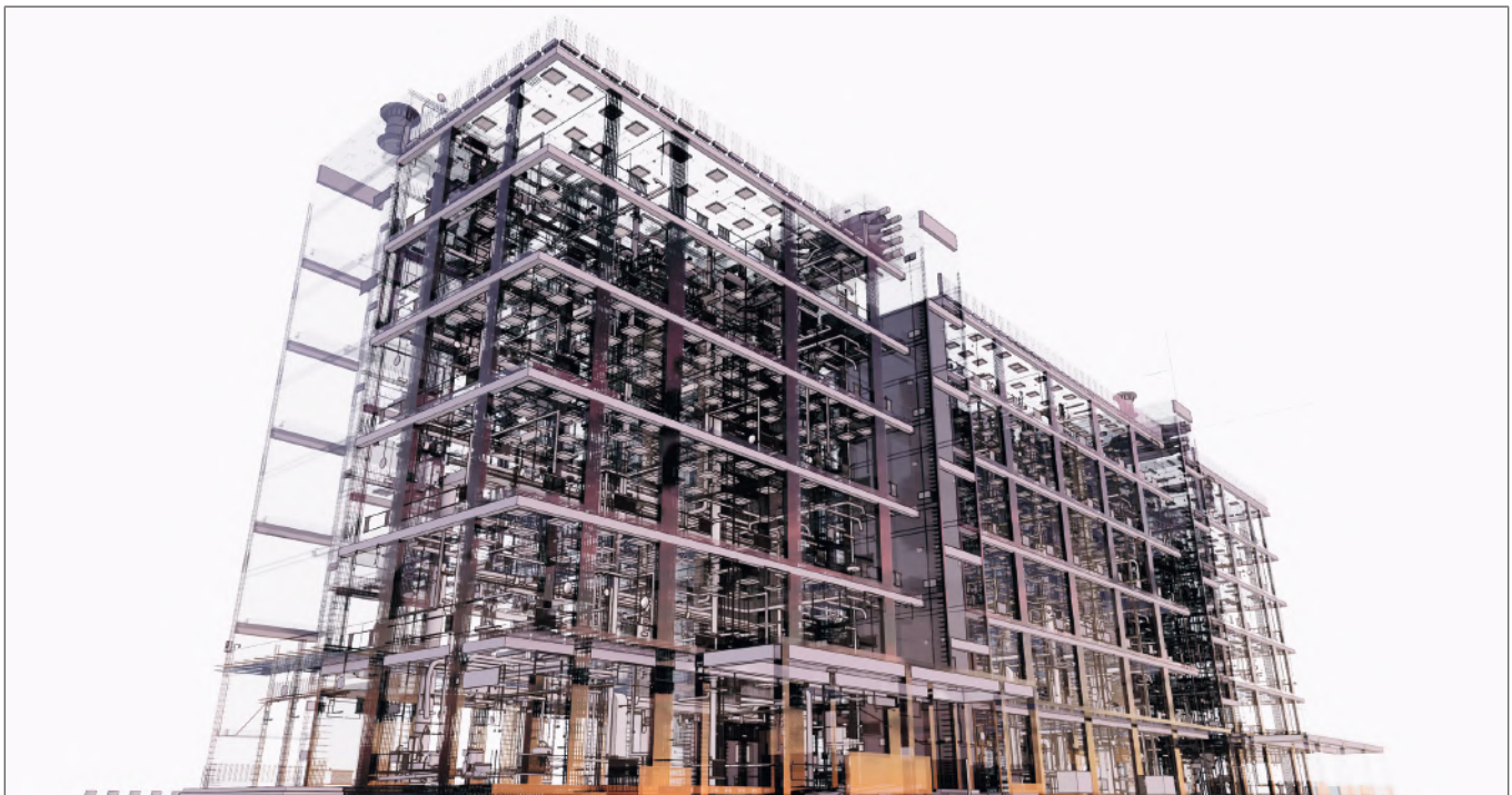
Figure 11: Visualisation of the BIM model of an office building (without the outer skin)
